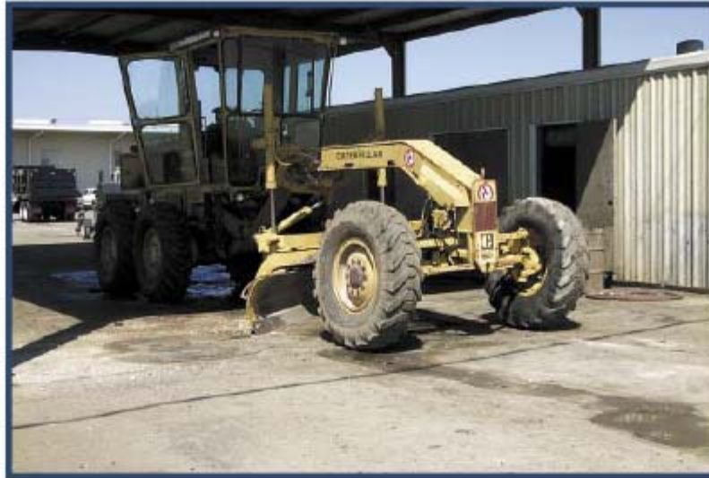
Figure 10. The wash area at this facility is large enough to accommodate the size of the heavy equipment being cleaned. However, this unit is placed too close to the edge of the wash area, allowing wash water to run off the pad.
