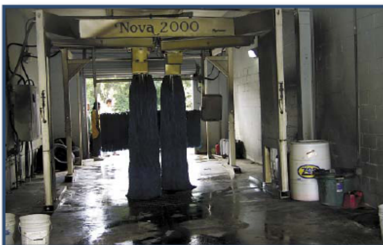
Figure 1. Example of a rollover car wash. The wash water is well confined inside the system. Also, no significant amount of rainwater is introduced into the system.
