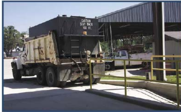
Figure 24. Pumpout truck used to remove the sludge from the settling tank at this facility.
